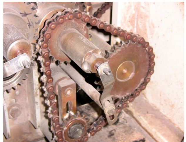
Chain drive on a card feedroll
