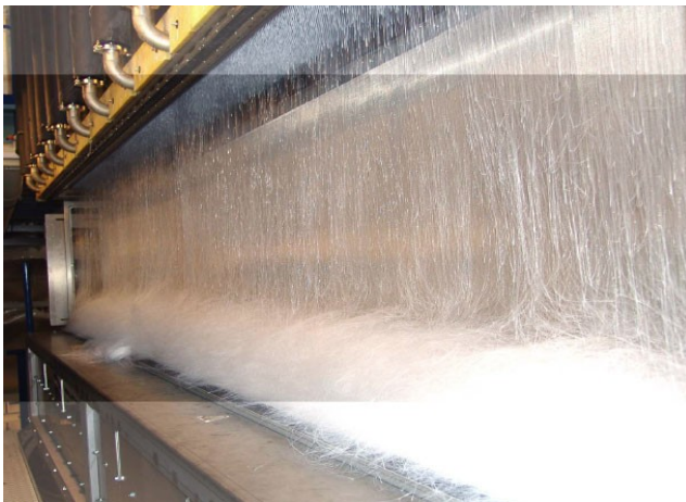
Filaments being collected on a Reifenhäuser spunbond machine
