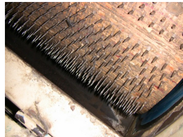
Pinned FO cylinder showing the pins imbedded in the wooden lagging
