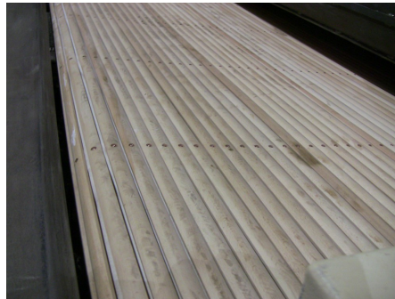
Apron with close spacing of the slats and rounded top slats
