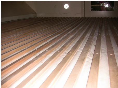
Apron with wide spacing and slats flat on one side
