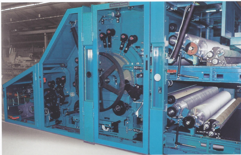
▲ SERVO-CARD SC 2-5 CC, Arbeitsbreite AB = 2.500 mm SERVO-CARD SC 2-5 CC, working width ww = 2.500 mm
